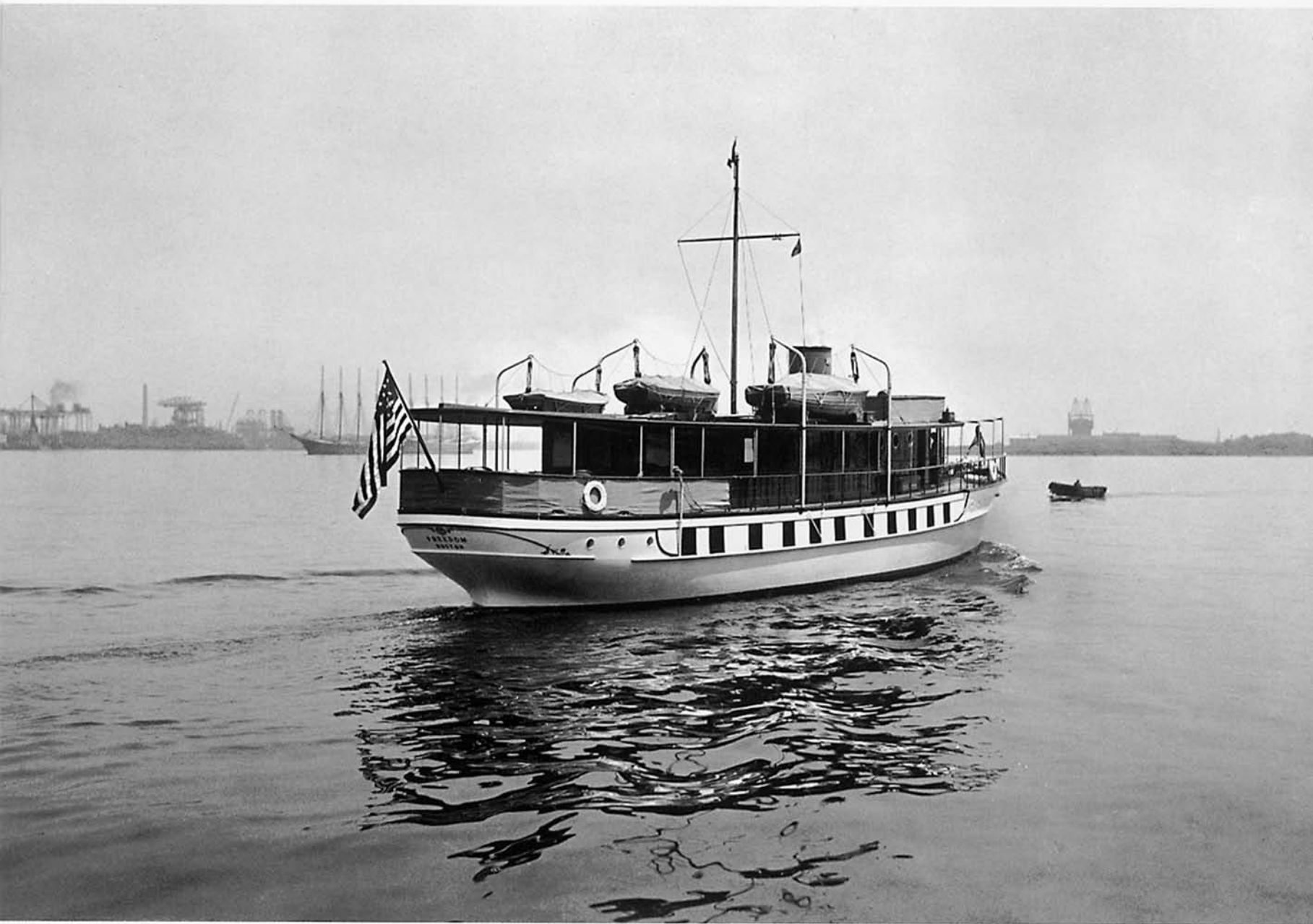
104 feet and built in 1926 for A. J. Fay. Designed and built by Mathis-Trumpy. Powered by a pair of gas 6-cylinder Wintons.
